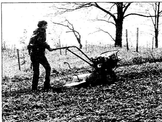
Photo 4-27: Tilling on a moderate slope. (Don't till on steep ground.)
